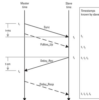
Fig. 6 - IEEE 1588 Synchronism Mechanism
