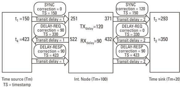
Fig 7 – Example of transparent clock with asymmetrical delays
