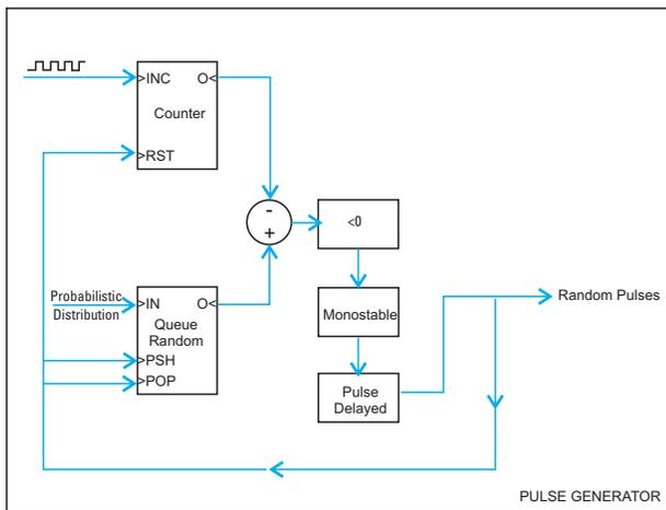
Fig. 10 - Random generation of pulses in the time scale of the model
