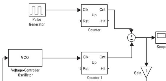
Fig. 4 - Model with Automatic Frequency Adjustment
