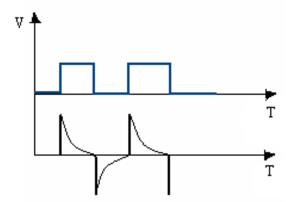
Fig. 8 Pulses for RC configuration derivative
