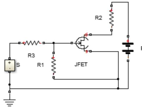
Fig. 2 Circuit for detecting atmospheric electricity
