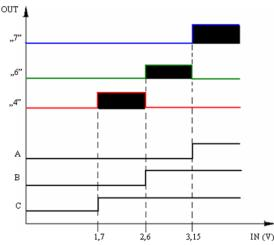
Fig. 7 Three levels of voltage from comparator
