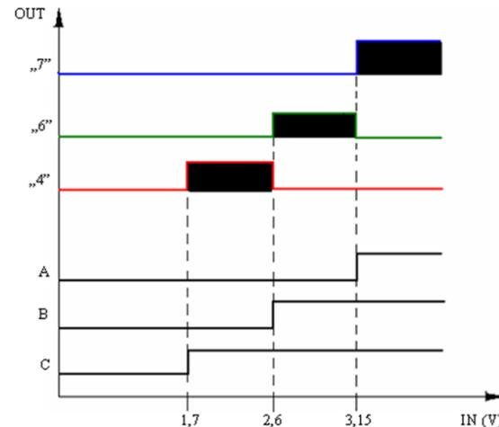
Fig. 7 Three levels of voltage from comparator
