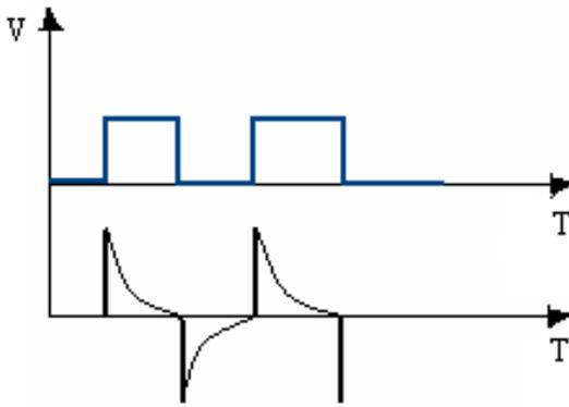
Fig. 8 Pulses for RC configuration derivative
