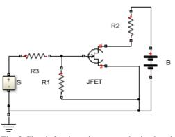
Fig. 2 Circuit for detecting atmospheric electricity
