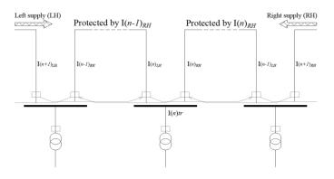
Fig. 4. System layout with the protection mechanism.
