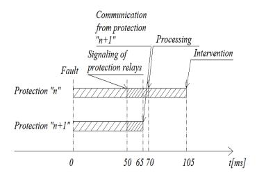
Fig. 6. Intervention times for the proposed logic.
