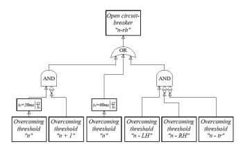
Fig. 5. Logic diagram of the nth digital protection.
