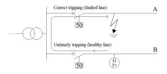
Fig. 12. Example of untimely tripping in a primary substation due to the massive presence of DG along the lines.
