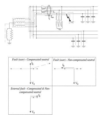
Fig. 7. Conditions for a ground fault, electrical scheme and phasor representation.
