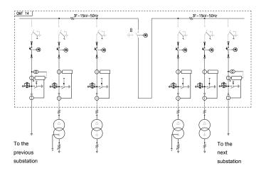
Fig. 3. Details of two secondary, consecutive MV/LV substations from the diagram in Fig.1.
