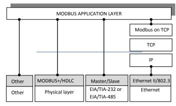
Fig. 11. Modbus communication stack.
