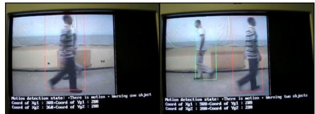
Fig. 9 Motion detection in RGB for two objects.
