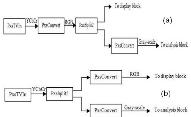
Fig. 3 Possible ways to do the conversion, (a) before splitting, (b) after splitting
