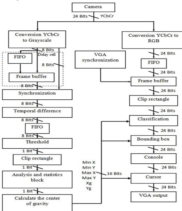
Fig. 6 Diagram of motion detection
