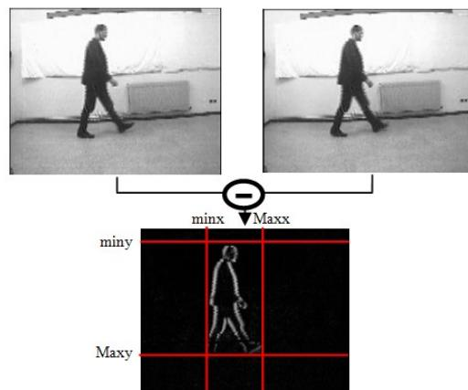
Fig. 5 Temporal difference and the Min and Max in X and Y axis
