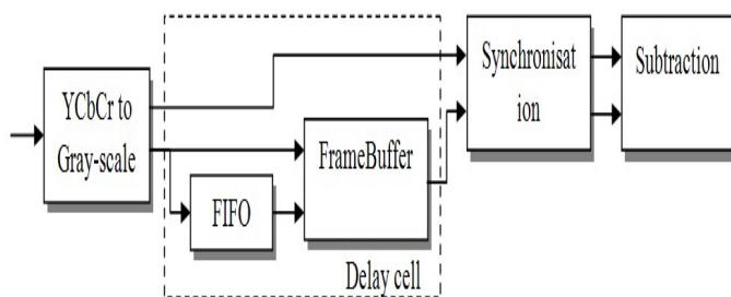
Fig. 4 The delay cell and difference diagram
