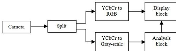
Fig. 2 Object detection process algorithmic basic block diagram
