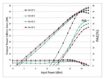
Fig. 10 Power performance versus drain bias  $V_{DS}$  for 0.6  $\mu m \times 8 \times 125 \ \mu m$  with  $L_{fp}$  0.5  $\mu m$  when measured at 8 GHz
