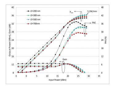
Fig. 8 Large-signal performance of the 0.6  $\mu$ m × 6 ×125  $\mu$ m with L<sub>fp</sub> = 0.2, 0.3, 0.5, and 0.7  $\mu$ m at 8 GHz. The device was biased with V<sub>ds</sub> = 35 V and V<sub>gs</sub> = -2.4 V
