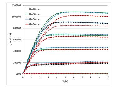
Fig. 5 Drain current-voltage ( $I_{DS}-V_{DS}$ ) characteristics of a 0.6 µm × 2 × 100 µm AlGaN/GaN HEMT with  $L_{fp} = 0.2, 0.3, 0.5, and 0.7$  µm. The gate bias was swept from -4 to 1 V in a step of 1 V
