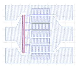
Fig. 1 Layout of the field-plated AlGaN/GaN HEMT structure
