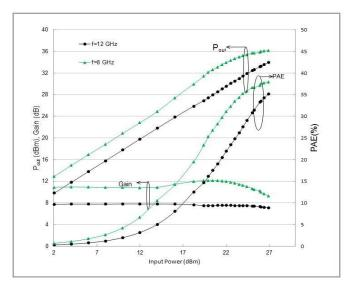
Fig. 12 Large-signal performance of the 0.6  $\mu$ m × 6 ×125  $\mu$ m with L<sub>fp</sub> = 0.5 $\mu$ m at 8 GHz and 12 GHz. The device was biased with V<sub>ds</sub> = 30 V and V<sub>gs</sub> = -2.4 V
