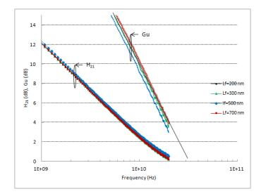
Fig. 7 Short-circuit current gain |h21| and unilateral power gain of a 0.6  $\mu$ m × 6 × 125  $\mu$ m AlGaN/GaN HEMT with L<sub>fp</sub> = 0.2, 0.3, 0.5, and 0.7  $\mu$ m. Device was biased at V<sub>DS</sub> = 25 V and V<sub>gs</sub> = -3.0 V
