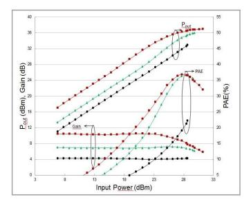
Fig. 11 Large-signal performance of the 0.6  $\mu$ m × 8 × 125  $\mu$ m with  $L_{fp}$  = 0.5 $\mu$ m at 8 GHz, 10 GHz and 12 GHz. The device was biased with  $V_{ds}$  = 30 V and  $V_{gs}$  = -2.4 V
