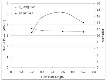
Fig. 9 Power performance versus length of field plate  $L_{fp}$  for devices of 0.6  $\mu$ m × 6 ×125  $\mu$ m when measured at 8 GHz with drain biases of 35 V
