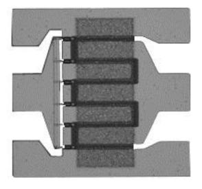
Fig. 4 Optical microscope image of fabricated 6×125µm HEMT
