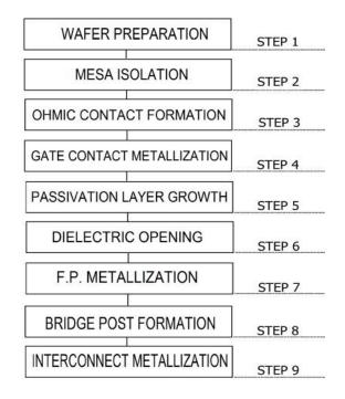
Fig. 3 Flow chart of GaN HEMT fabrication process including field plate step
