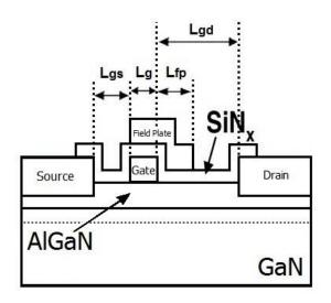
Fig. 2 Schematic of field-plated AlGaN/GaN HEMT structure
