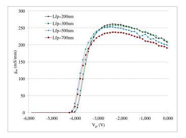
Fig. 6 Transcoductance  $(g_m - V_{gs})$  characteristics of a 0.6  $\mu$ m × 2 × 100  $\mu$ m AlGaN/GaN HEMT with L<sub>fp</sub> = 0.2, 0.3, 0.5, and 0.7  $\mu$ m
