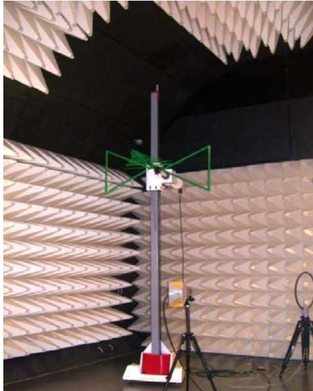
Fig. 4. Semianechoic chamber for measuring EMI and EMS testing, Tomas Bata University in Zlín
