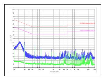
Fig. 3. The result of measurement of electromagnetic interference on the line terminals according to EN 55022 ed. 3, Article 5.1.
