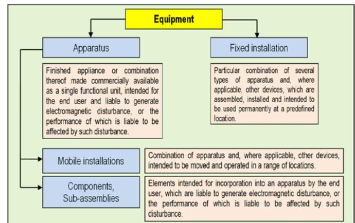
Fig. 2: Basic definitions of terms in the field of the requirements for EMC products [5] (modified Valouch, 2013)
