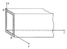
Fig. 6 schematic representation of an electromagnetic waveguide.
