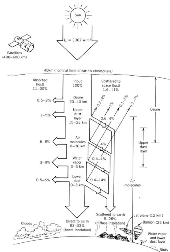
Fig. 1 Nominal range of clear sky absorption and scattering of incident solar energy[12].
