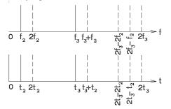
Fig. 1. Responses of nonlinear systems to multisignal excitation: above - responses of the nonlinear circuit to a series of harmonic excitations, below - responses of the nonlinear resonant medium to the excitation in the form of delta functions.
