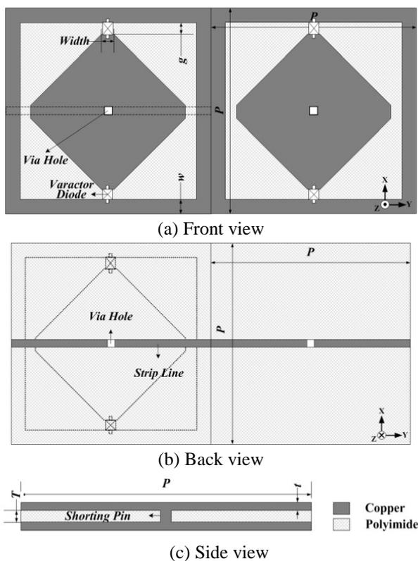
Fig. 1. Designed unit cell of the reconfigurable FSS
