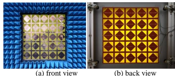
Fig. 3. Fabricated reconfigurable FSS ;
