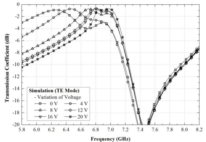
Fig. 2. Simulated transmission results of the proposed reconfigurable FSS for different bias voltages : TE mode,
