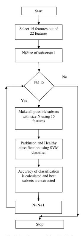
Fig. 2 Algorithm to get highest classification accuracy.
