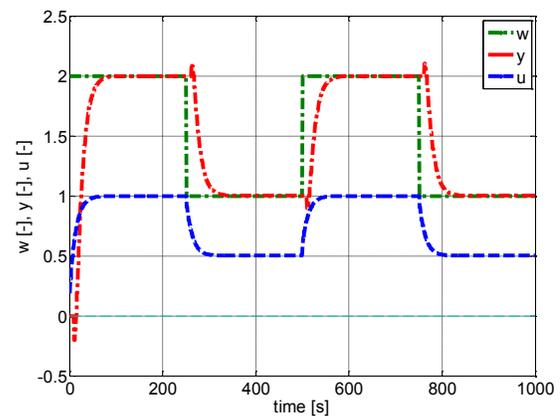
Fig. 19 Control of nominal model  $G_{N_3}(z^{-1}), K = 2$
