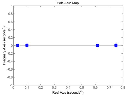
Fig. 11 Pole map of control nominal model  $G_{N3}(z^{-1})$
