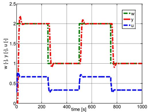
Fig. 14 Control of perturbed model  $G_{\Delta P1}(z^{-1})$  -  $K = 3$
