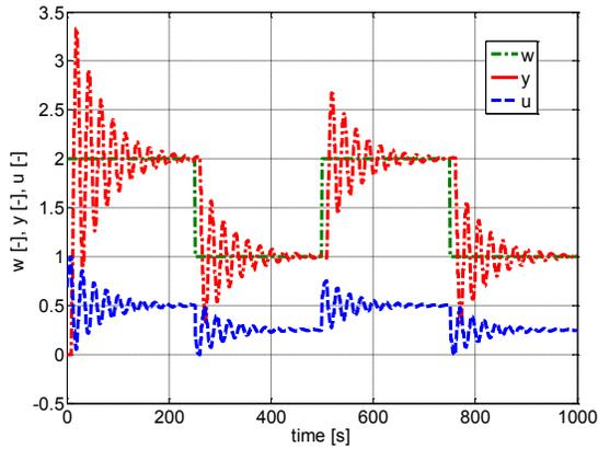
Fig. 6 Control of perturbed model  $G_{p2}(z^{-1})$ ,  $K = 4$
