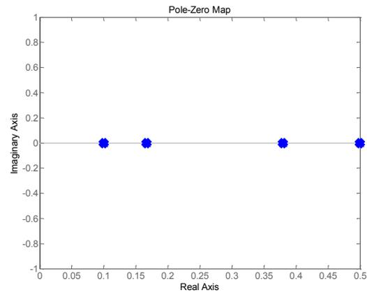
Fig. 4 Pole map of control nominal model  $G_{N1}(z^{-1})$
