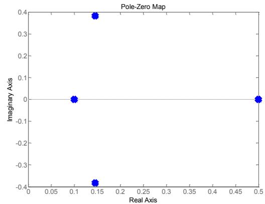
Fig. 9 Pole map of control nominal model  $G_{N2}(z^{-1})$
