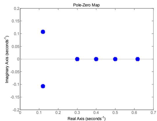
Fig. 20 Pole map of control nominal model  $G_{N_3}(z^{-1})$
