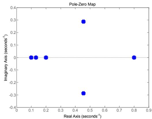
Fig. 13 Pole map of control nominal model  $G_{N1}(z^{-1})$
