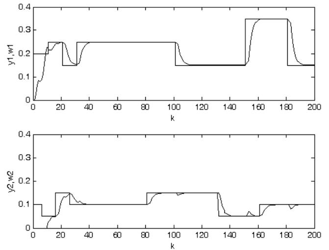
Fig. 3 Adaptive control with discrete controller
