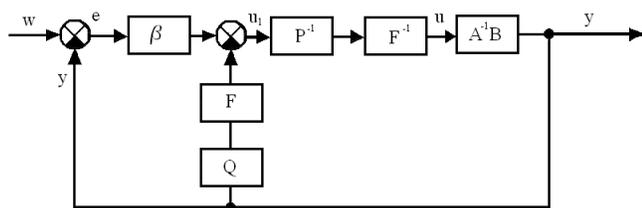
Fig. 1 Block diagram of 2DOF configuration
