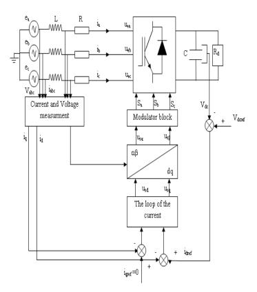
Fig.4. Basic block of the VOC scheme.
