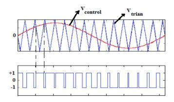
Fig.3. Description of bipolar PWM modulation
