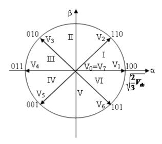
Fig.2. Voltage vectors generated by the rectifier
