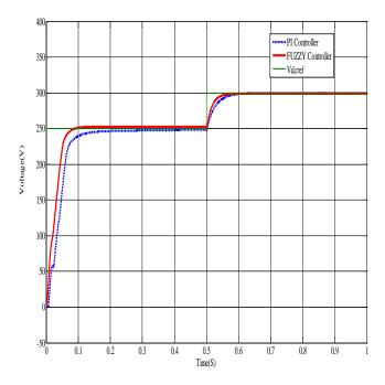
Fig.11. Control system step response  $(V_{dcref} = 250 \text{ to } 300 \text{ V})$
