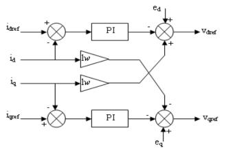
Fig .5. Decoupled controller
