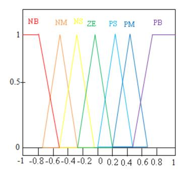
Fig .8 Membership functions of the error
