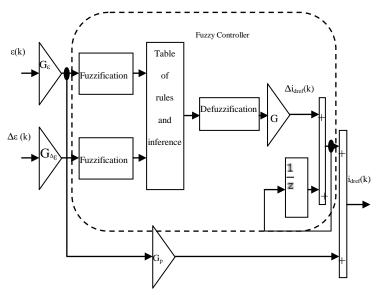
Fig .7. DC voltage regulation with FUZZY controller
