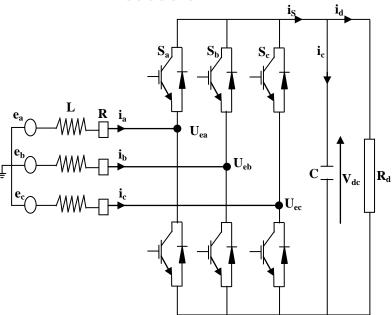
Fig.1. General Diagram of the PWM rectifier
