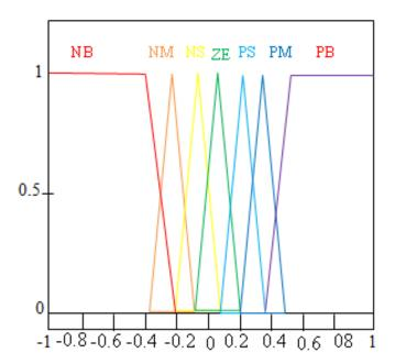
Fig .10. Membership functions of the output
