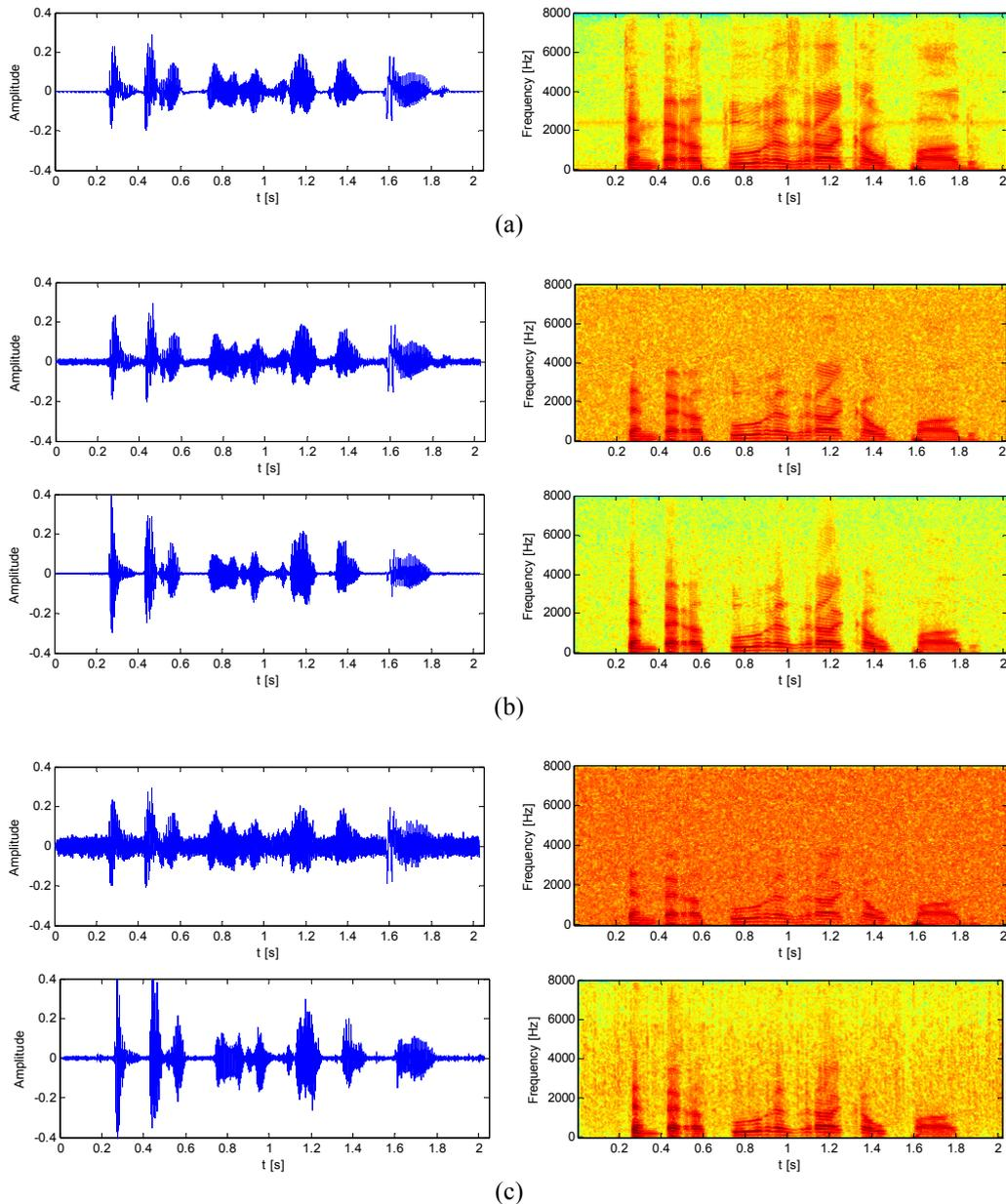
Fig. 3 Noise reduction example: (a) clean speech and its spectrogram; (b) noise reduction for SNR=10dB – top panels noisy speech and its spectrogram, bottom panels noise reduced speech and its spectrogram; (c) noise reduction for SNR=0dB – top panels noisy speech and its spectrogram, bottom panels noise reduced speech and its spectrogram
