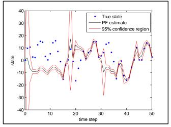
Fig. 3 PF estimates compared with true state
