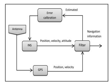
Fig. 1 Block diagram of loosely-coupled GPS/INS system.
