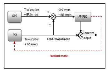
Fig. 3 Proposed approach in GPS/INS integration.
