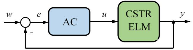
Fig. 7 Control system with CT external linear model.
