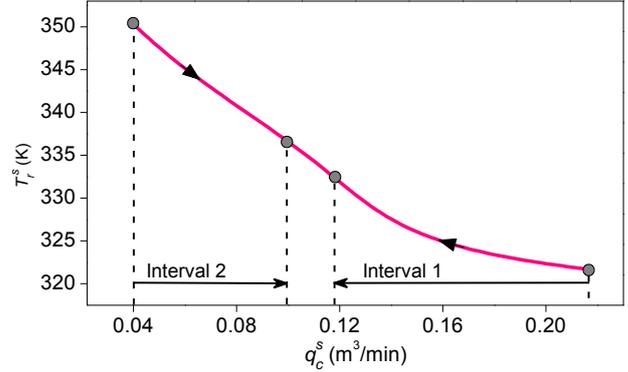
Fig. 6 Dependence of the reactant temperature on the coolant flow rate in the steady-state.
