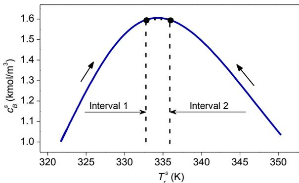
Fig. 2 Steady-state dependence of the product  $B$  concentration on the reactant temperature.
