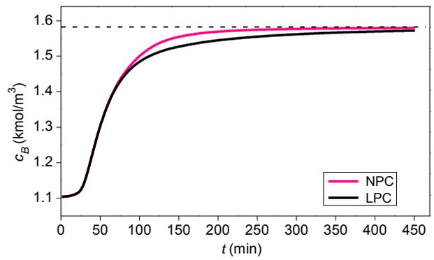
Fig. 12 Concentration  $c_B$  responses ( $K_w = 0.12$ ,  $G_w = 1.645$ ,  $t_s = 8$ ).
