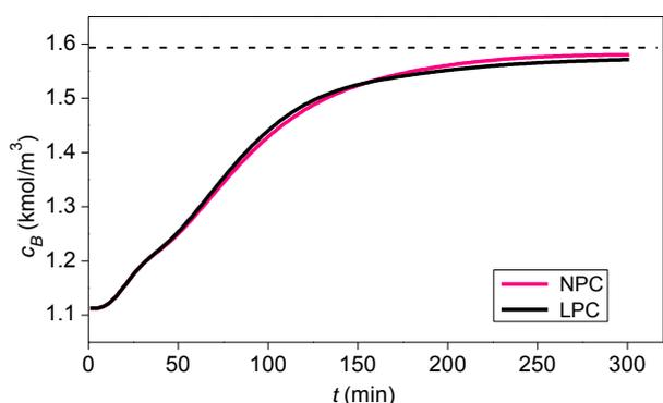
Fig. 17 Concentration  $c_B$  responses ( $K_w = 0.1$ ,  $G_w = -2.206$ ,  $t_s = 8$ ).
