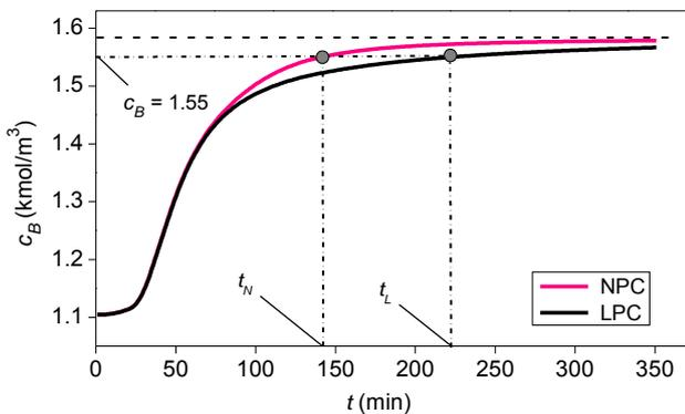
Fig. 10 Concentration  $c_B$  responses ( $K_w = 0.15$ ,  $G_w = 2.05$ ,  $t_s = 10$ ).
