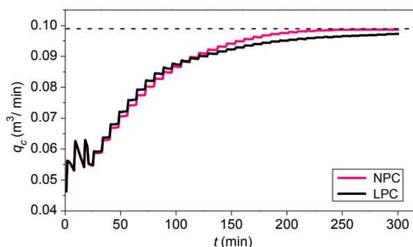
Fig. 18 Coolant flow rate courses ( $K_w = 0.1$ ,  $G_w = -2.206$ ,  $t_s = 8$ ).
