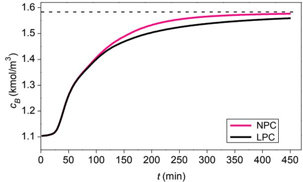
Fig. 14 Concentration  $c_B$  responses ( $K_w = 0.12$ ,  $G_w = 1.645$ ,  $t_s = 12$ ).
