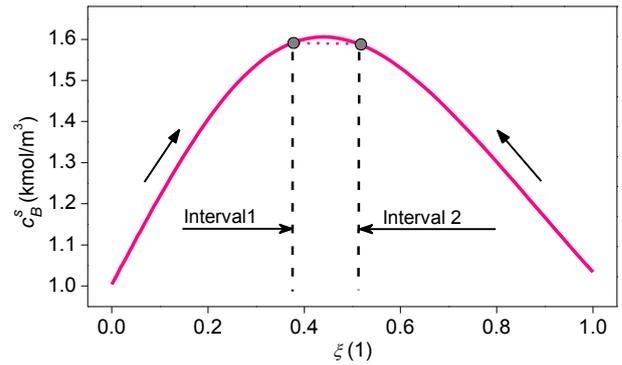
Fig. 3 Steady-state dependence of component  $B$  concentration on transformed reactant temperature.
