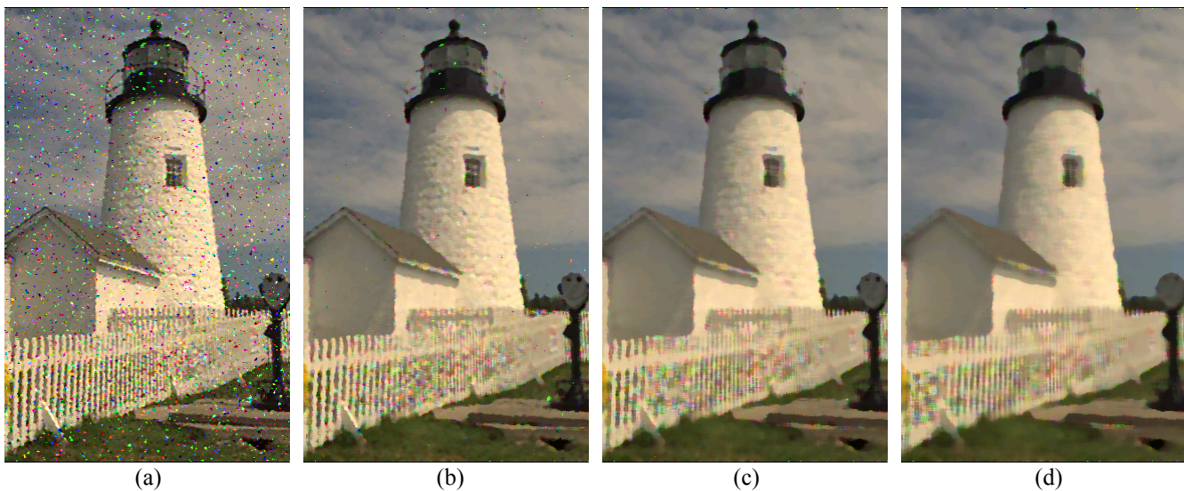
Fig.5 – Portion of the “Lighthouse” image corrupted by impulse noise with probability 0.4 and processed by (2N+1)\times(2N+1) scalar median filters: (a) N=1 , (b) N=2 , (c) N=3 , (d) N=4 .
