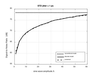
Fig. 4. Ratio between the sine wave amplitude *A* and the STD  $\sigma_{|c_1|}$  of jitter noise within the sine-wave frequency bin as a function of *A*.
