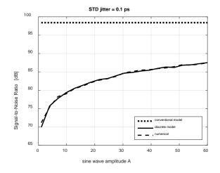
Fig. 5. Same as Fig. 4 but with jitter STD equal to 0.1 ps.
