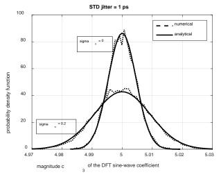
Fig. 10. Probability density function of the magnitude  $|c_3|$  of the DFT coefficient corresponding to the input waveform consisting in a sine wave and a third harmonic. The noise-free case and the case  $\sigma_n = 0.2$  are reported in the figure.
