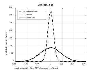
Fig. 2. Probability density function of the imaginary part  $b_1$  of the DFT coefficient corresponding to the input sine wave having amplitude 10 and phase  $\pi/3$ .
