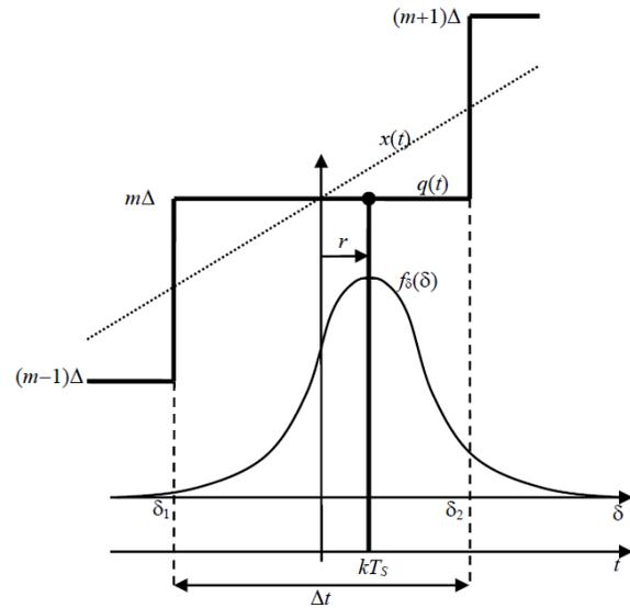
Fig. 1. Quantized version  $q(t)$  of the input signal  $x(t)$ , and definition of the probabilistic quantities related to the sampling instant  $kT_s$ .
