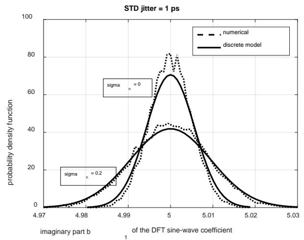
Fig. 8. Probability density function of the imaginary part  $b_1$  of the DFT coefficient corresponding to the input waveform consisting in a sine wave and a third harmonic. The noise-free case and the case  $\sigma_n = 0.2$  are reported in the figure.
