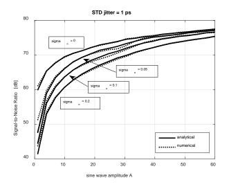
Fig. 6. Ratio between the sine wave amplitude *A* and the STD  $\sigma_{|c_1|}$  of jitter noise within the sine-wave frequency bin as a function of *A* and for different levels of additive Gaussian noise.
