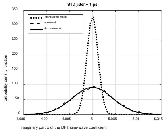
Fig. 2. Probability density function of the imaginary part  $b_1$  of the DFT coefficient corresponding to the input sine wave having amplitude 10 and phase  $\pi/3$ .
