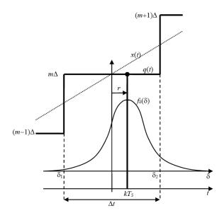
Fig. 1. Quantized version q(t) of the input signal x(t), and definition of the probabilistic quantities related to the sampling instant  $kT_{\rm S}$ .
