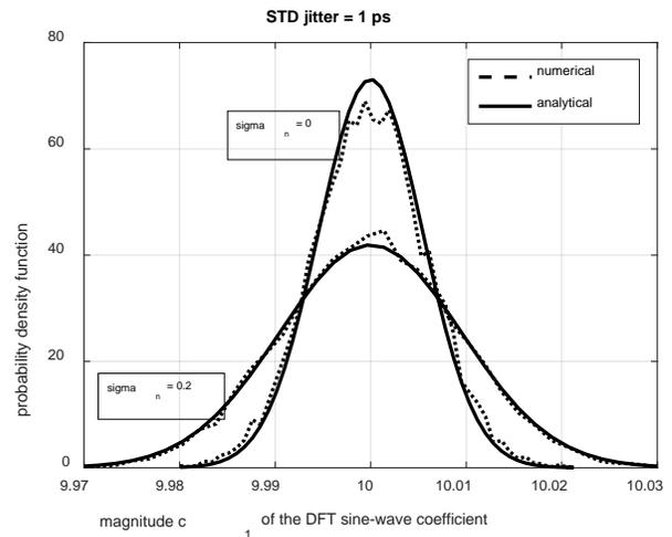
Fig. 9. Probability density function of the magnitude  $|c_1|$  of the DFT coefficient corresponding to the input waveform consisting in a sine wave and a third harmonic. The noise-free case and the case  $\sigma_n = 0.2$  are reported in the figure.
