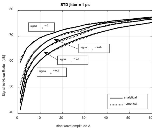
Fig. 6. Ratio between the sine wave amplitude  $A$  and the STD  $\sigma_{|c_1|}$  of jitter noise within the sine-wave frequency bin as a function of  $A$  and for different levels of additive Gaussian noise.
