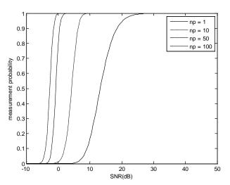
Fig. 4. Measurement probability under Swerling IV
