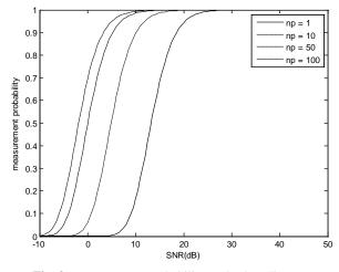
Fig. 3. Measurement probability under Swerling III
