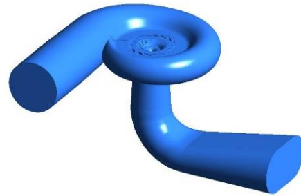
Fig. 1. Computational domain of full channel of Francis turbine
