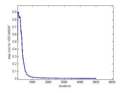
Fig. 5 Step size curve for the VSS-IMSAF.
