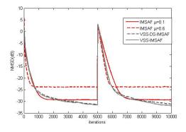
Fig. 7 NMSD curves of the IMSAF, VSS-IMSAF and VSS-DS-IMSAF for system sudden change
