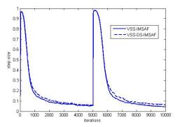
Fig. 8 Step size curves of the VSS-IMSAF and VSS-DS-IMSAF for system sudden change
