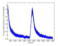
Fig. 9 Average number of selected subband of the VSS-DS-IMSAF for system sudden change.
