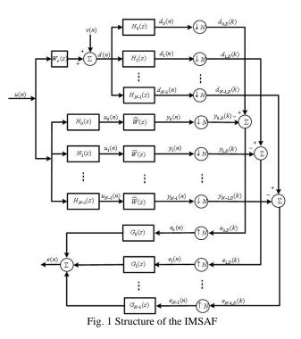
Define the input signal matrix  $\mathbf{U}(k)$ , the desired signal vector  $\mathbf{d}_D(k)$ , the estimated signal vector  $\mathbf{y}_D(k)$ , the subband noise vector  $\mathbf{v}_D(k)$  and the error signal vector  $\mathbf{e}_D(k)$  as follows
