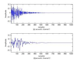
Fig. 6 Measured room acoustic impulse response.
