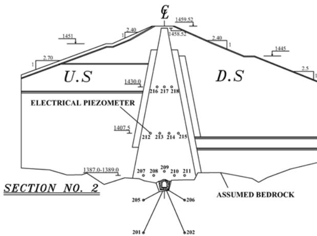
Fig. 1. Piezometers' position of cross section No. 2.
