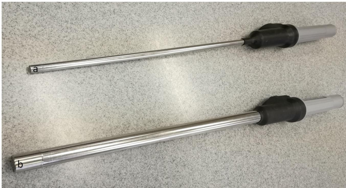
Fig. 1. MTEC tactile mechanoreceptor with 7 sensors (a) and 19 sensors (b).
