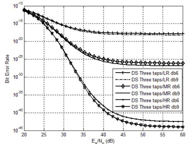
Fig. 7 BER performance versus  $E_s/N_o$  for the three service rates using *db6* and *db9* wavelet packets.
