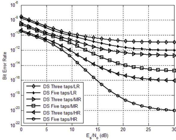
Fig. 4 BER performance versus  $E_s/N_o$  for the three service rates using the DS3 and DS5
