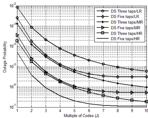
Fig. 11 Effect of multiple number of codes on  $P_{out}$
