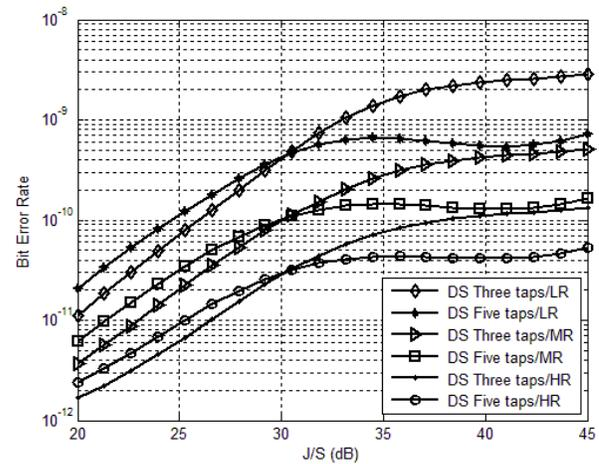
Fig. 9 Effect of  $\mathfrak{I}/S'$  and filter taps on BER for the three service rates
