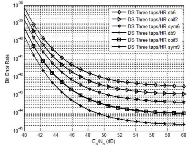
Fig. 6 BER performance versus  $E_s/N_o$  for three WPs family and two filter lengths for each one of them
