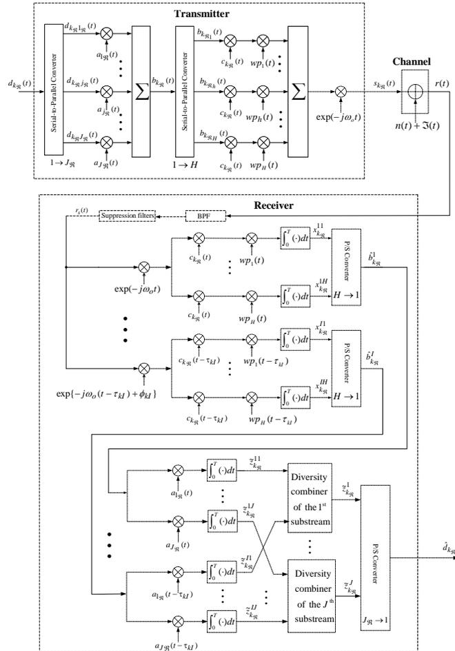
Fig. 1 WP-MC\MCD-CDMA system with multirate and SF
