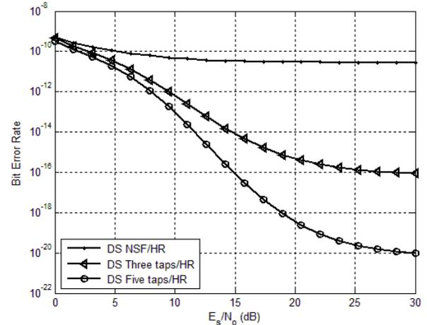
Fig. 2 BER performance versus  $E_s/N_o$  for HR service with and without SF
