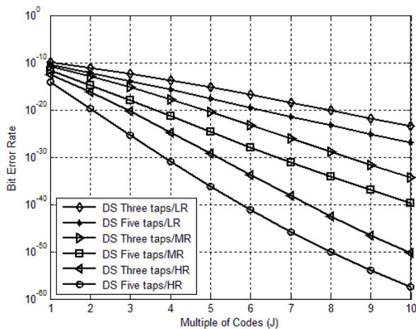
Fig. 10 Effect of multiple number of codes on BER
