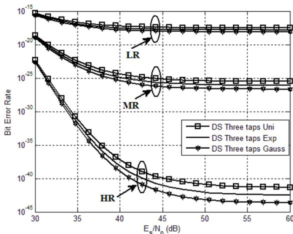
Fig. 8 Effect of MIP on BER performance for the three service rates
