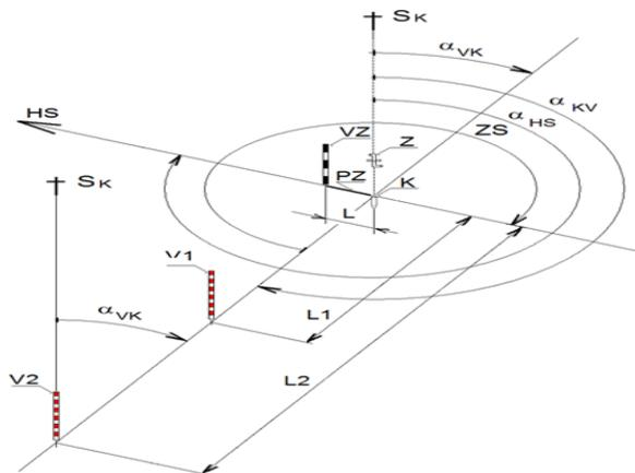
Fig. 3 Aiming the cannon into main direction of shooting (HS) while stakes are not in the HS
