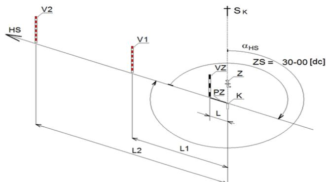
Fig. 1 Placement of stakes for aiming into HS in front of the cannon
