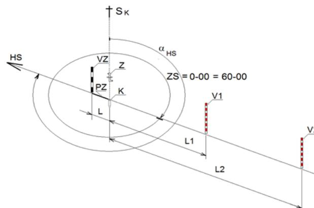
Fig. 2 Placement of stakes for aiming into HS behind the cannon
