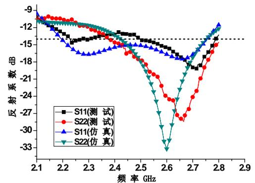
(a) Reflection coefficient of proposed antenna
