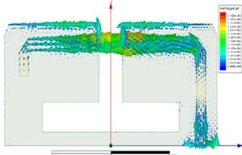
(b) Simulated current vector on conventional feed structure of port 1
