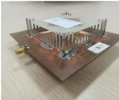
(a) Fabrications of antenna element
