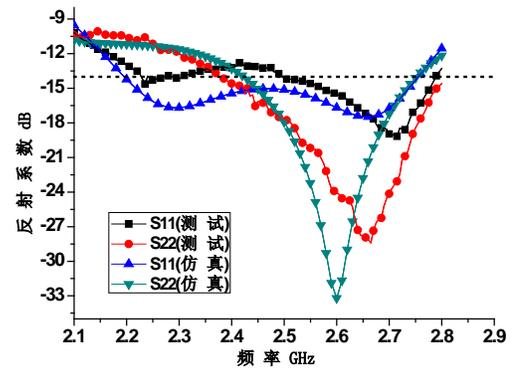
(a) Reflection coefficient of proposed antenna
