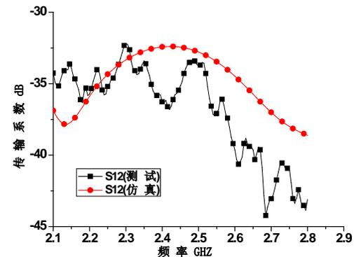
(b) Transmission coefficient of proposed antenna
