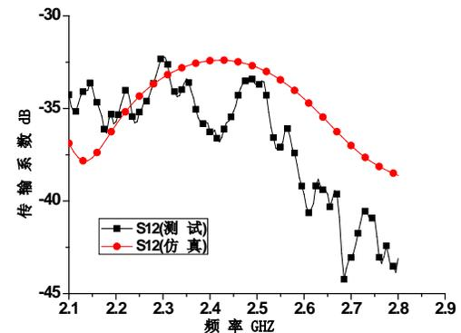
(b) Transmission coefficient of proposed antenna
