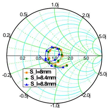
(b) Simulated impedance curve of proposed antenna versus different position of  $\Gamma$  shape strip
