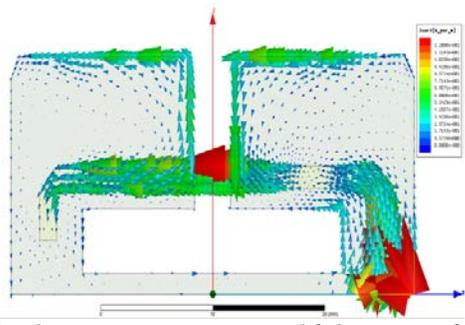
(a) Simulated current vector on proposed fed structure of port 1
