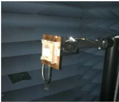
(b) Test antenna installed at test gauge in anechoic chamber room
