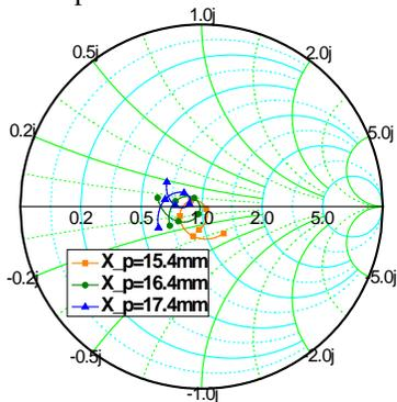
(a) Simulated impedance curve of proposed antenna versus different length of upper slot
