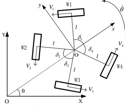
Fig. 1. Wheel placement of mobile robot
