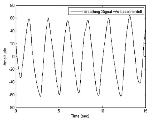
Fig. 7 Respiratory signal after removing the baseline-drift artifact
