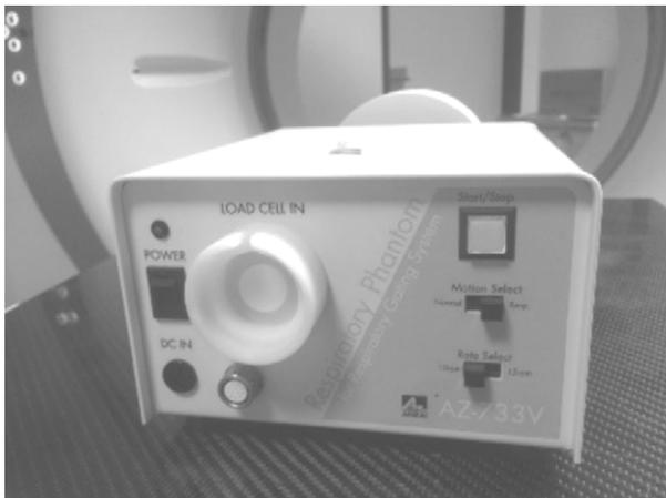
Fig. 1 Respiratory phantom used in experiment
