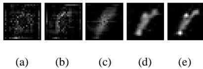
Fig.5 the kernel estimation in the solving process: (a) result in the 1<sup>st</sup> iteration; (b)result in the 3<sup>rd</sup> iteration; (c) result in the 6<sup>th</sup> iteration; (d)result in the 9<sup>th</sup> iteration; (e) final estimated kernel
