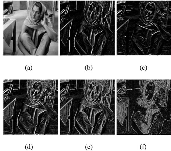
Fig.1 (a) “barbara” image; (b) image gradients in horizontal direction; (c) image gradients in vertical direction; (d) image gradients extracted by total variation method; (e) image gradients extracted by the method in [4]; (f) image gradients extracted by Laplacian operator
