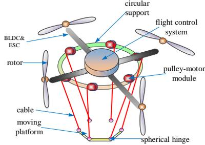
Fig. 1. Structure diagram of a flying cable driven parallel robot
