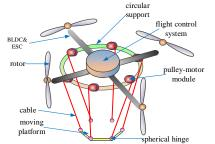
Fig. 1. Structure diagram of a flying cable driven parallel robot
