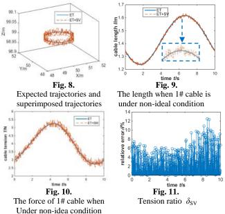
*C.* Effect of four rotor unmanned aerial vehicle on cable tension
