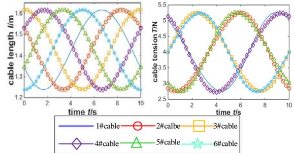
Fig. 7. Variation of cable length and cable tension in compound trajectory
