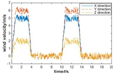
Fig. 5. Wind speed along X, Y, Z direction
