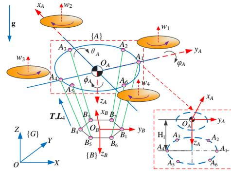
Fig. 2. Kinematic model of a flying cable driven parallel robot
