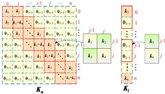
Fig. 4. Cable local frame system total stiffness matrix assembly process
