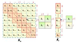
Fig. 4. Cable local frame system total stiffness matrix assembly process
