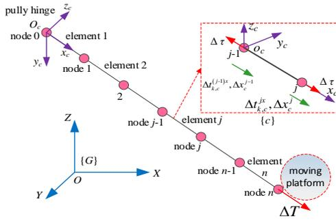
Fig. 3. Cable discretization model
