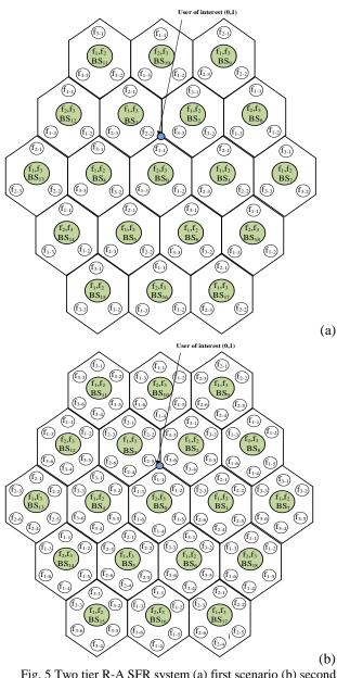
Fig. 5 Two tier R-A SFR system (a) first scenario (b) second scenario
