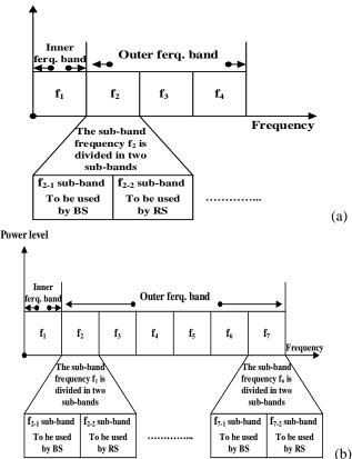
Fig. 4 frequency allocation for (a) first scenario (b) second scenario
