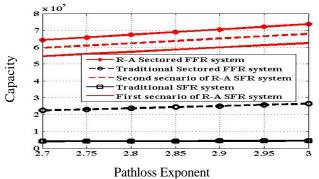
Fig. 9 Capacity variation against PL exponent for different interference mitigation systems
