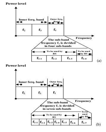
Fig. 6 Frequency allocation for (a) first scenario (b) second scenario
