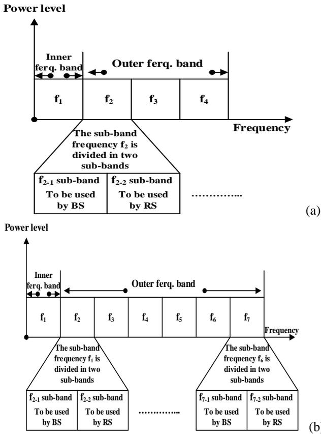
Fig. 4 frequency allocation for (a) first scenario (b) second scenario
