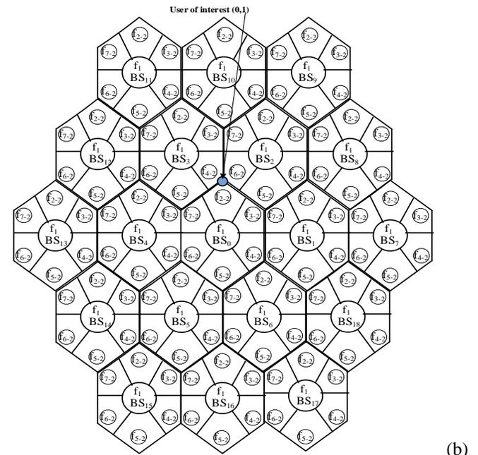
Fig. 3 two tier relay assisted sectored FFR system (a) first scenario (b) second scenario
