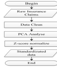
Fig. 2. Data preprocessing flowchart
