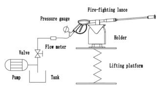
(b) Fig. 1 Structure of the experiment system
