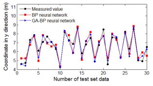
(b) Comparison of the landing position in the y direction Fig. 3 Comparison of the predicted and measured landing positions of the water jet
