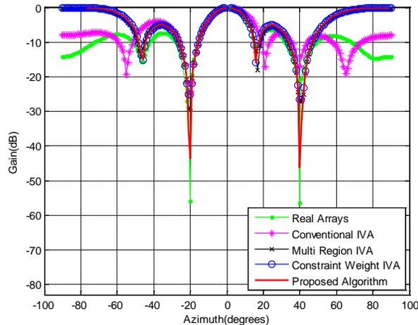
Fig.7 Analysis beamforming under burst interference
