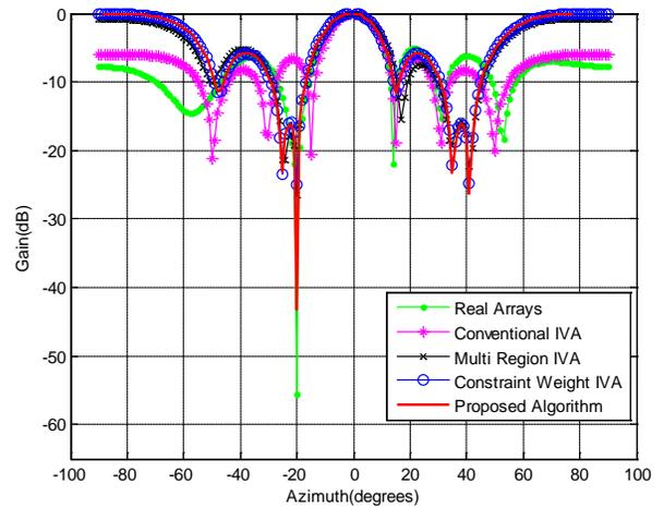
Fig.5 Analysis beamforming under large transformation angle
