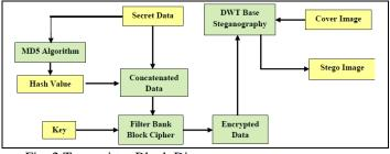
Fig. 2 Transmitter Block Diagram
