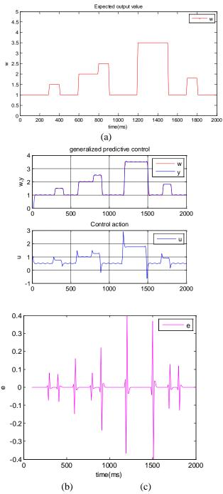
Fig. 6. Response results of velocity control in step disturbance
