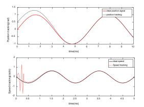
Fig. 9 the angle tracking trajectory and speed tracking trajectory of sliding-mode control
