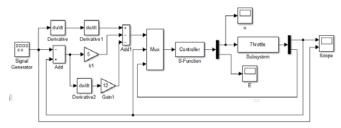
Fig. 7 the electric throttle control system model
