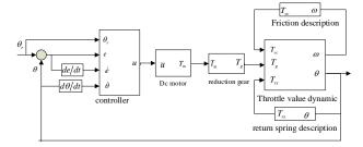
Fig. 3 the equivalent structure diagram of electronic throttle
