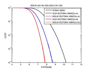
Fig. 7 PAPR performance of SLM ISC-FDMA MIMO schemes with Nt=2, N=256 and M=128.
