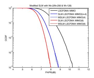
Fig. 6 PAPR performance of SLM LSC-FDMA MIMO schemes with Nt=2, N=256 and M=128.
