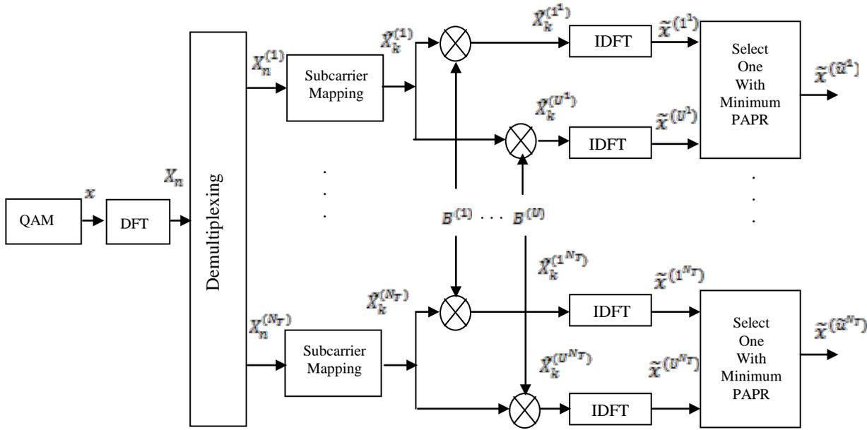
Fig. 3 Block diagram of modified SLM SC-FDMA MIMO uplink system.
