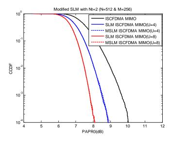
Fig. 5 PAPR performance of SLM ISC-FDMA MIMO schemes with Nt=2, N=512 and M=256.
