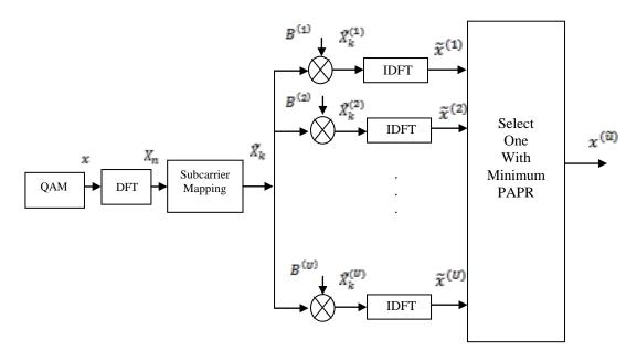
Fig. 1 Block diagram of SISO SLM SC-FDMA uplink system.
