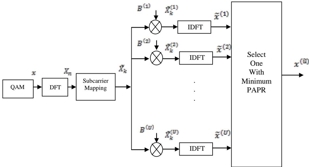
Fig. 1 Block diagram of SISO SLM SC-FDMA uplink system.
