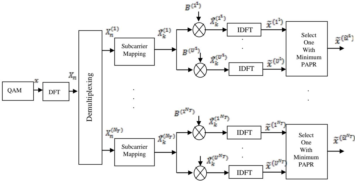
Fig. 2 Block diagram of SLM SC-FDMA MIMO uplink system.
