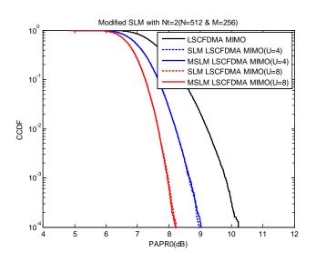
Fig. 4 PAPR performance of SLM LSC-FDMA MIMO schemes with Nt=2, N=512 and M=256.
