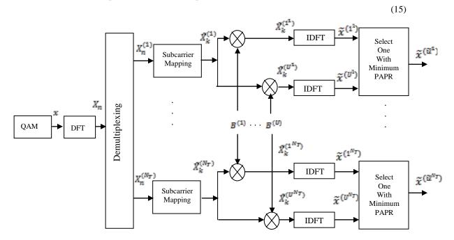
Fig. 3 Block diagram of modified SLM SC-FDMA MIMO uplink system.
