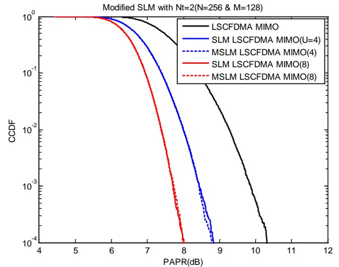
Fig. 6 PAPR performance of SLM LSC-FDMA MIMO schemes with  $N_t=2$ ,  $N=256$  and  $M=128$ .
