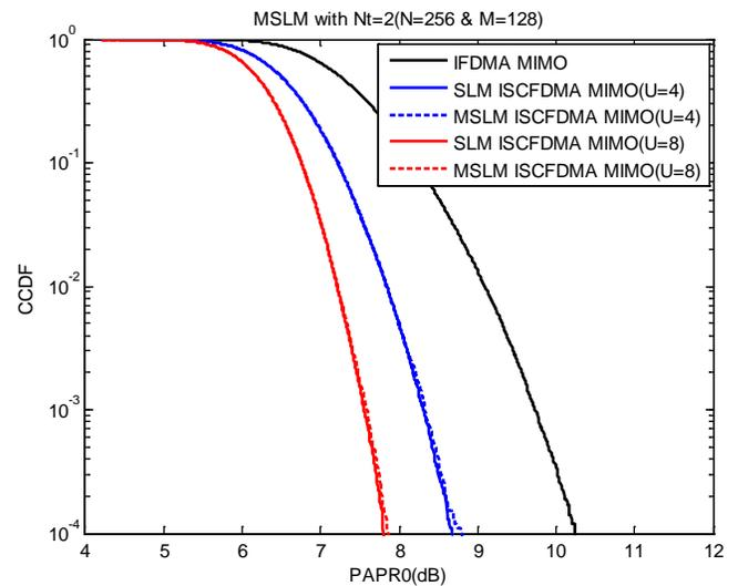
Fig. 7 PAPR performance of SLM ISC-FDMA MIMO schemes with  $N_t=2$ ,  $N=256$  and  $M=128$ .
