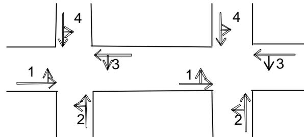
**Fig.1** A diagram of phase, two continuous connected intersections on the main road
