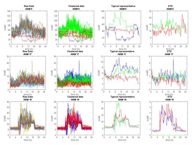
Fig. 8: Example of clustering of an industry consumer (high load).
