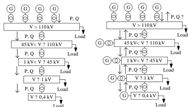
Fig. 1 Power system: Conv. (left), DEG (right) [1]
