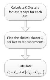
Fig. 11: Flow chart of Clustering based algorithm
