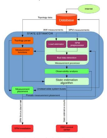
Fig. 2: State estimation block diagram [8]
