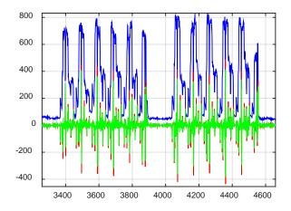
Fig. 10: Actual measurements (blue) and error (green, red) of estimated value (kW) for AMI# 6
