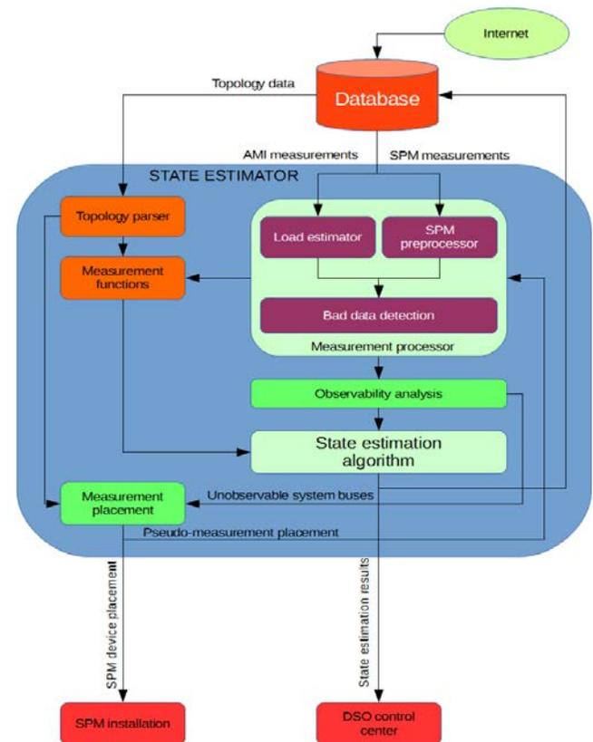
Fig. 2: State estimation block diagram [8]
