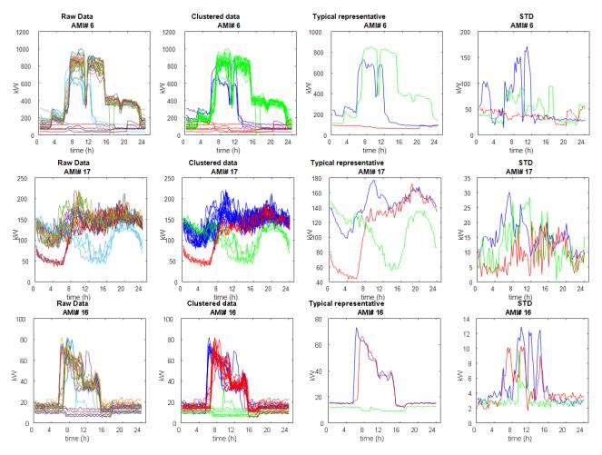
Fig. 6: Example of clustering of an industry consumer (high load).
