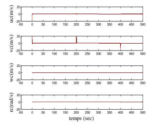
Fig.14 Virtual velocity using Bio-inspired Neurodynamics model (black solid line) and the backstepping method (red dashed line).
