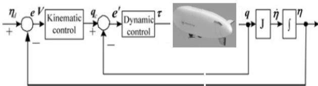
Fig.4 The cascaded controller of Airship.
