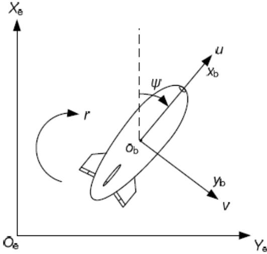
Fig. 2 Airship motion in the horizontal plane.
