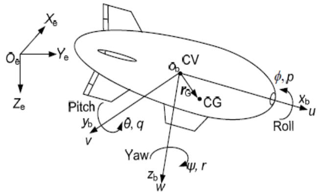
Fig. 1 Position of frames.
