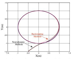
Fig.7.Systems trajectories using Bio-Inspired Neurodynamics model (black line) and the backstepping method (red dashed line).
