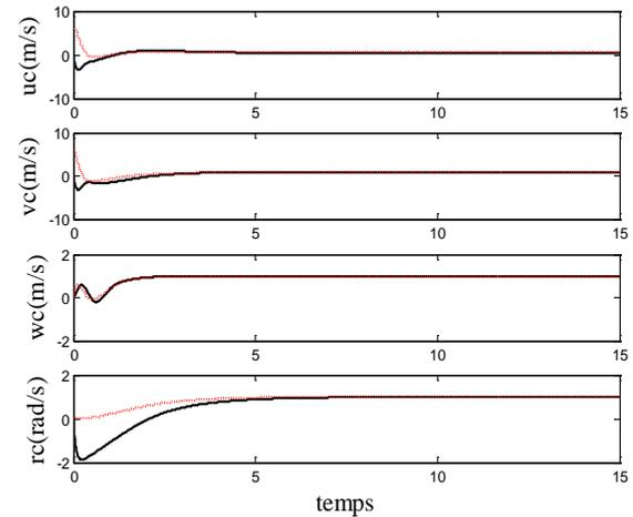
Fig.8. Virtual velocity using Bio-Inspired Neurodynamics model (black solid line) and the backstepping method (red dashed line).
