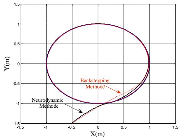
Fig.7. Systems trajectories using Bio-Inspired Neurodynamics model (black line) and the backstepping method (red dashed line).
