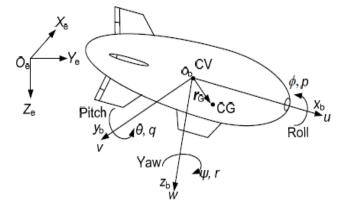
Fig. 1 Position of frames.
