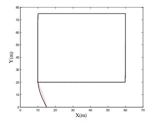
Fig.12 Systems trajectories using bio-inspired Neurodynamics model (black solid line) and the backstepping method (red dashed line).
