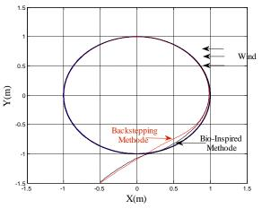
Fig.9. Systems trajectories using Bio-Inspired Neurodynamics model (black line) and the backstepping method (red dashed line) with inaccurate parameters and disturbances.
