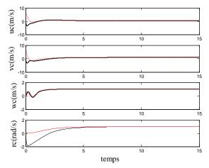
Fig. 10 Virtual velocity using Bio-Inspired Neurodynamics model (black solid line) and the backstepping method (red dashed line) with inaccurate parameters and disturbances.
