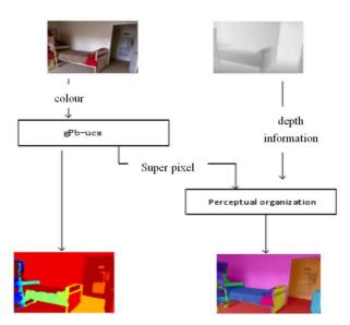
Fig. 3. Segmentation algorithm framework based on RGB-D indoor scene
