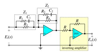
Fig. 2 analog lead-lag compensator
