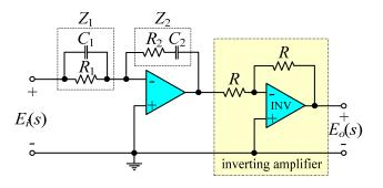
Fig. 3 analog PID controller
