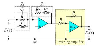
Fig. 4 analog PIDA controller
