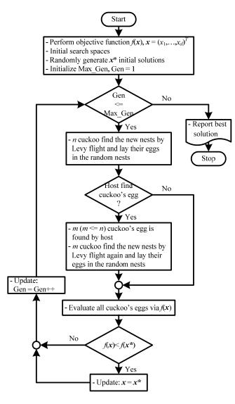
Fig. 1 flow diagram of CS algorithms
