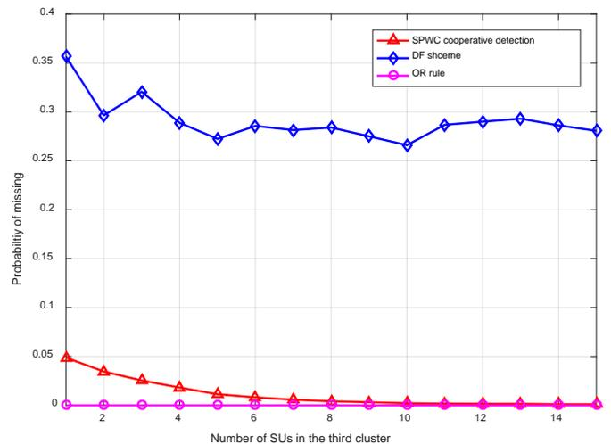
**Fig. 6.** Probabilities of missing with different cooperative users under the average SNR,  $\bar{\gamma}_2 = -13dB$
