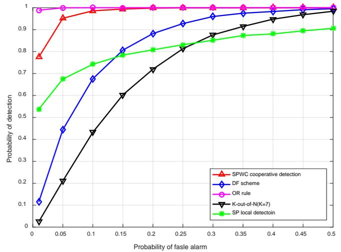
Fig. 2. Probabilities of detection under the average SNR,  $\bar{\gamma}_2 = -13dB$
