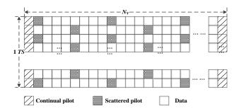
**Fig. 1.** The subcarrier positions of continual pilots, scattered pilots and data of CMMB signals in one time slot (1TS)
