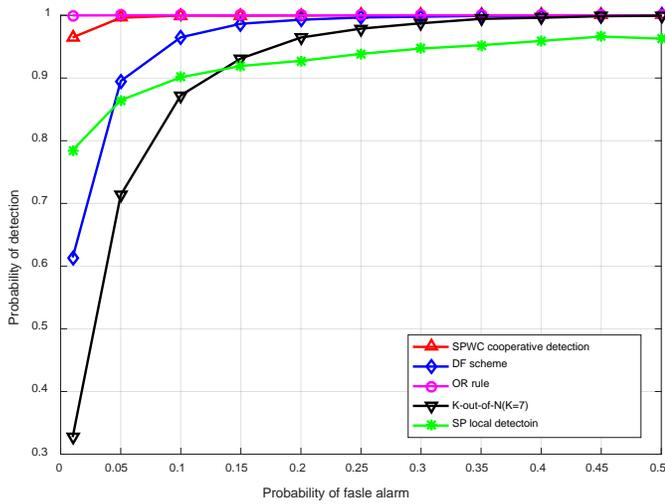
**Fig. 3.** Probabilities of detection under the average SNR,  $\bar{\gamma}_2 = -11dB$
