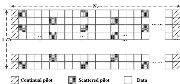
**Fig. 1.** The subcarrier positions of continual pilots, scattered pilots and data of CMMB signals in one time slot (1TS)
