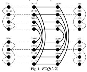
**Theorem 1**[11] .The degree of V(ECQ(s,t)) whose bit addresses end in 0 is s+1, while the degree of V(ECQ(s,t)) whose bit addresses end in 1 is t+1.
