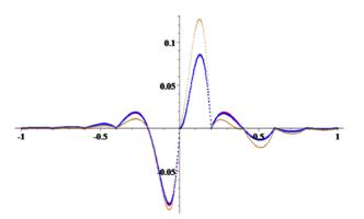
Fig.8. The errors of approximation of the function  $1/(1 + 25x^2)$  on the uniform grid (n = 10, h = 0.2).
