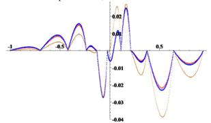
Fig.7. The errors of approximation of the function  $1/(1 + 25x^2)$  on the non-uniform grid (n = 10).
