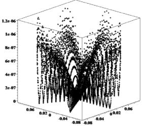
Fig. 19: Plot of the errors of approximation of the real part of function  $u(\rho, \varphi) = \sin(\rho e^{I\varphi})$  with splines (4), n=100, m=100.
