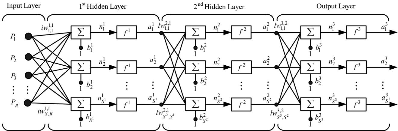
Fig. 4. Back propagation with two hidden layers
