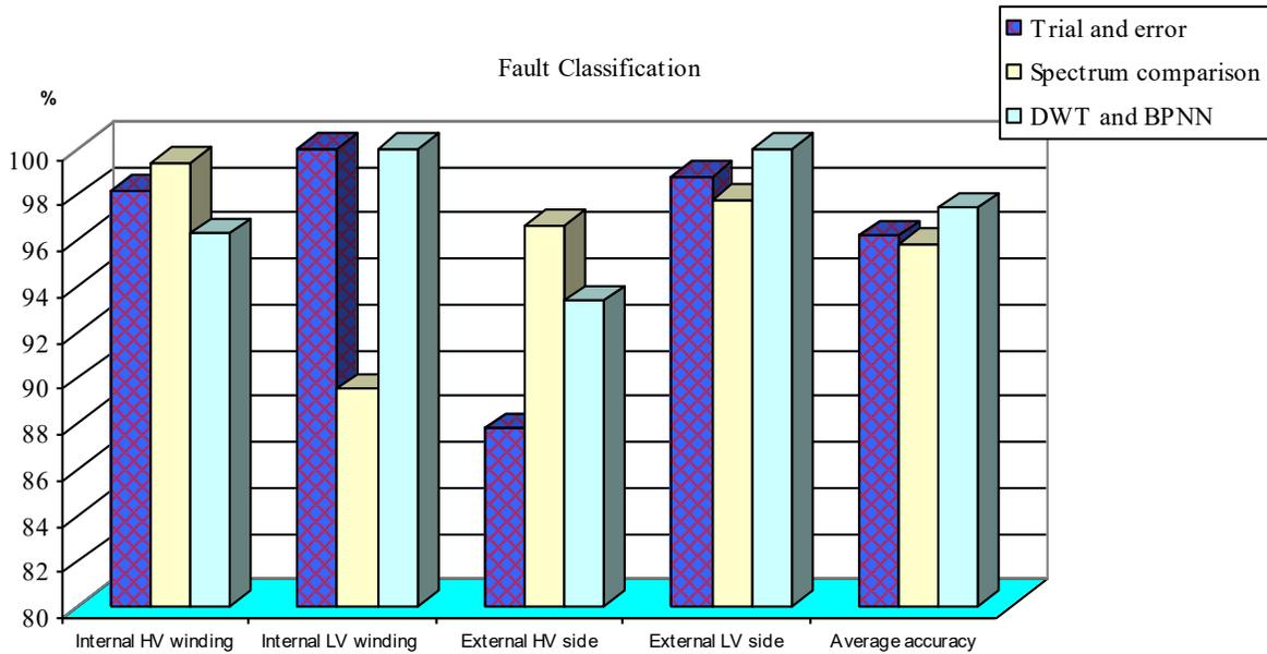
Fig. 5. Comparison of average accuracy for fault detection.
