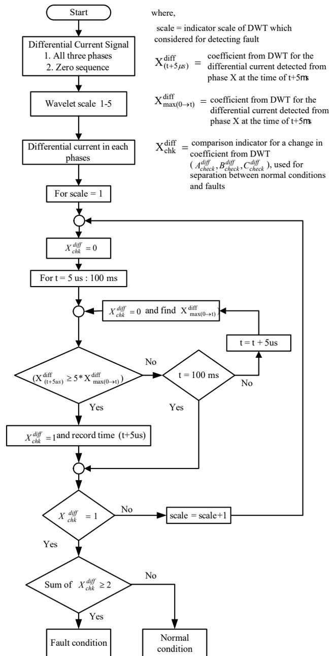
Fig. 3. Flowchart for detecting the fault condition
