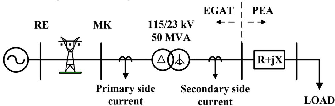
Fig. 1. The power transformer under studies [13].
