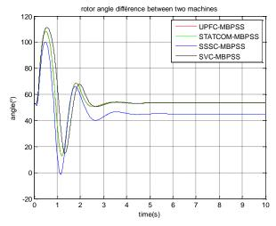
Fig. 19. Rotor angle difference between two machines
