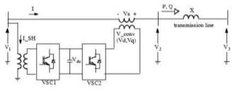
Fig. 4. Unified power flow controller
