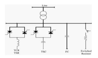
Fig. 2. Static VAR Compensator of SVC
