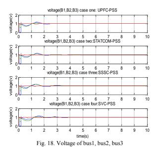
E. Simulation result for three phase fault using FACTS-MBPSS
