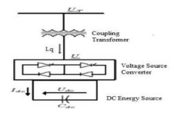
Fig. 3. Static Synchronous Compensator (STATCOM)
