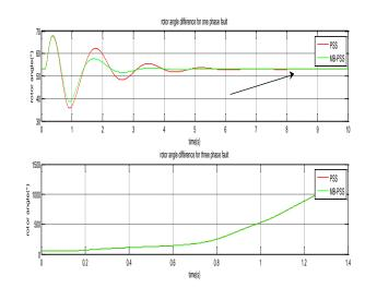
Fig. 23. Rotor angle difference between two machines in case of one phase fault and three phase fault respectively
