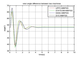
Fig. 12. Rotor angle difference between two machines
