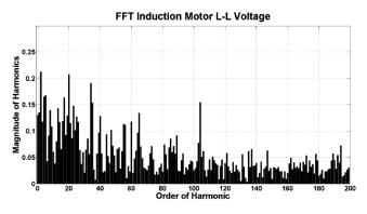
Fig.21. Harmonics of motor line-to-line voltage
