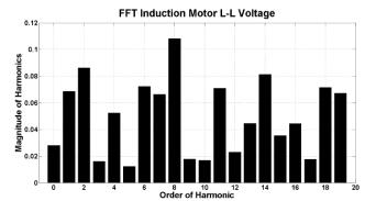
Fig.18. Harmonics of motor line-to-line voltage
