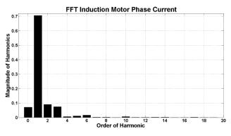
Fig.19. Harmonic of motor phase current
