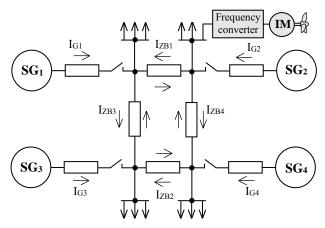
Fig.1. Scheme of investigated ship's power system
